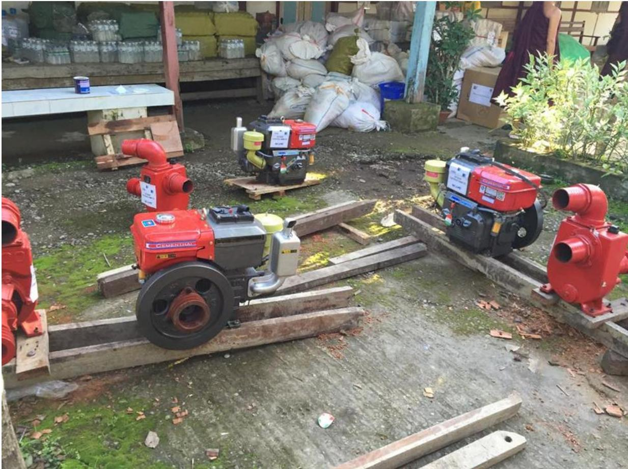
Water pumps to drain the contaminated reservoirs.
